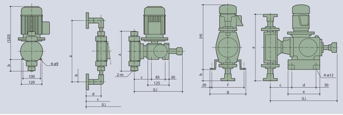
Note: All illustrations above show "PVC" type. The suction flange made of SUS is straight
